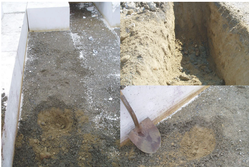
Figure 2. Soil and EPS-blocks at Løkkeberget. Left and bottom right pictures: EPS-blocks (1989) and soil profile 0-20cm. Top right picture: Reference soil profile 0-140 cm (Photo: Tor Helge Johansen, NPRA, year 2006)
